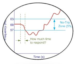
loss of renewable source or a fault. The figure on the left shows common  $\pm$  5% limits where frequency should remain at all times. A system operating at 60 Hz should remain bounded to 57-63 Hz despite contingencies. Falling outside these boundaries would trip the frequency-protection and cause a total system blackout (i.e., an unstable condition).
