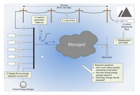
In the event of contingencies, the diesel units can serve the entire city and restore service in under 20 minutes. However, what is desired is to reduce the dependence on diesel and operate a single, under-sized diesel generator in parallel with the renewable resources.
