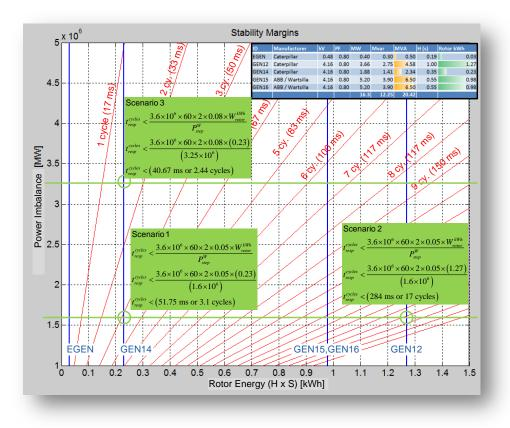
single diesel unit. The vertical axis represents the step-change of power under an assumed contingency. The
